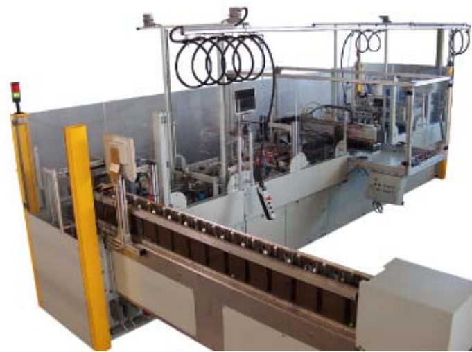
PM 25/50 Pass personalization system with chip programming
