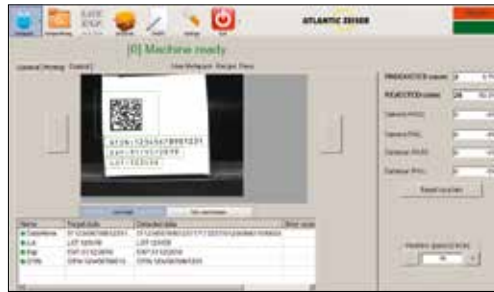
The setup of recipes and the control of all functions is managed over an intuitive graphical user interface. The inspection camera triggers if necessary the rejection and reports every activity to the MEDTRACKER database. In addition all audit-relevant information and events are exchanged as well.
