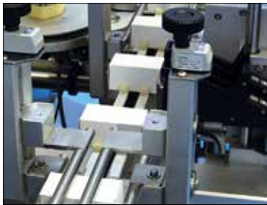
The elaborate transport belt guarantees best and reproducible coding results at any time. Format changes can be managed in little time while the printer and camera position can be swapped on demand.
