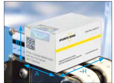
The optionally available tamper-evident module allows to seal cartons with labels and reliably checks their presence. Format changes for boxes with flaps in different opening directions can be realized in little time. Format range (A x B x H) in moving direction: min. 30 x 15 x 60 mm, max. 240 x 140 x 200 mm
