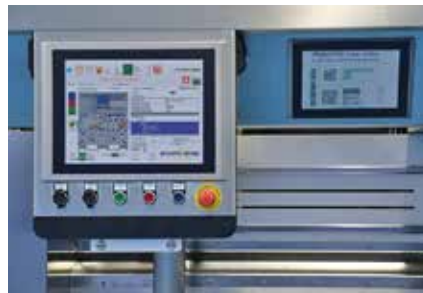
The high resolution inspection camera can be easily set up over an intuitive user interface. The camera accurately checks content and quality of code and text elements. On demand all results can be directly reported to the database of the Unique Code Software.
