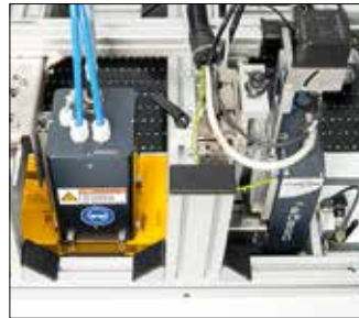
The OMEGA DoD inkjet technology guarantees consistent high print quality thanks to UV curing inks resistant against wear, water and solvents.
